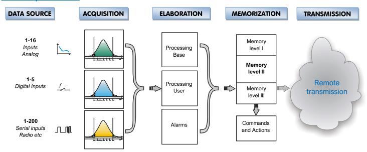
Acquisition capacity: evolution has an acquisition capacity of signals practically unlimited, tied only to available physical and logical connections. With a basic equipment that involves interfacing 1÷16 analog inputs, 1÷5 digital inputs, 2 RS232 serials, 1÷200 RS485 or SDI12 serial devices, USB, Lan network, wireless, IoT, I2CBus, ModBus, radio, etc., it is difficult to imagine anything more versatile.
