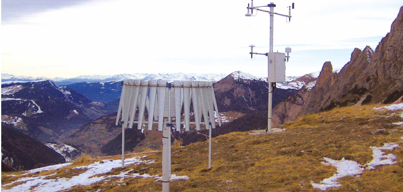
Example of installation with "Single Alter" shielding system for heated rain gauge, according to WMO (Gardena Valley - Italy), together with standard AWS
