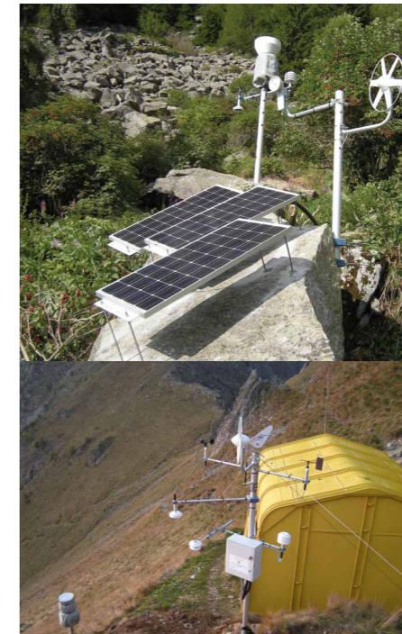
Automatic weather station in Bivacco Festa (2320 m), at the head of Rabbia Valley (Sonico, BS - Italy), equipped with low consumption heated rain gauge with thermal insulator
